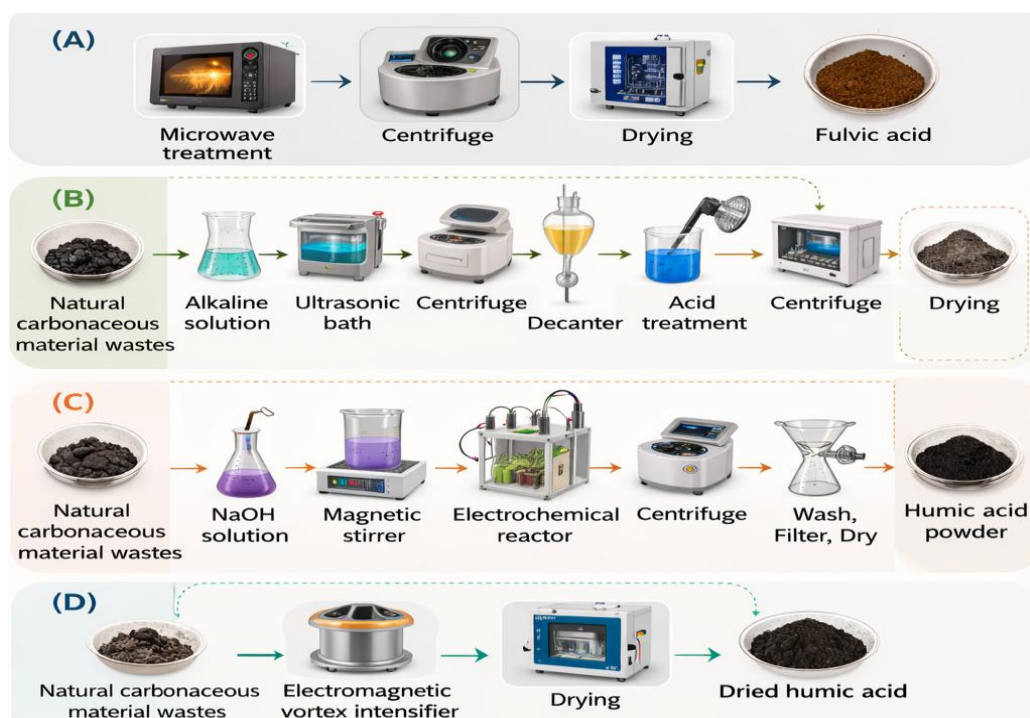
Figure 2 – Production of HA from natural carbonaceous materials using process intensification methods: (A) microwave-assisted extraction using H 2 O 2 ; (B) integration of ultrasound with oxidizing agents; (C) combined ultrasonic treatment and extraction; (D) application of an electromagnetic vortex activator with ferromagnetic particles.
